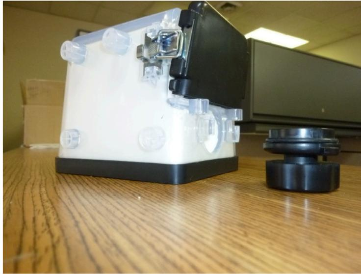
3. Release both (left and right) toggle latches from the catch plates in order to remove the front window.
