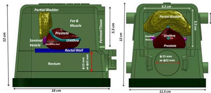
Internal tissues setup of the Brachytherapy prostate phantom. Diameter of 15 mm or 22 mm according to client demand.
