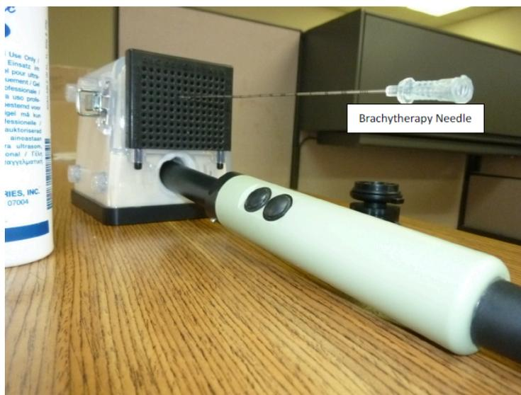
7. Insert the brachytherapy needle through the template holes and follow up its path using the ultrasound planes (Transverse or Sagittal). Probe Brachytherapy Needle
